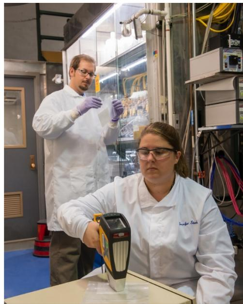
Argonne scientists test the utility of a handheld X-Ray Fluorescence instrument for prescreening Environmental Swipe Samples
